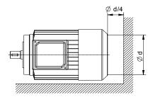
For constructions with shaft end upwards the user must prevent liquid entry from the shaft!
