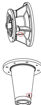
**Note: If the seal ring between the Gear Box and the intermediate casing/bell housing adaptor is fully efficient, there should be no oil in the intermediate casing.**
