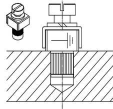
*Install Gear Box casings in compliance with local installation regulations. Ensure that the casing is earthed with the earthing clamps supplied. To earth Geared Motors, use the earth screws provided on the motors.*
