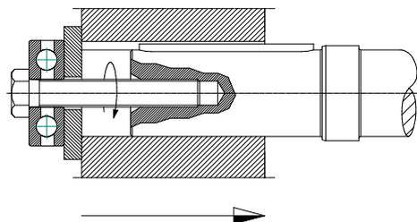
*To mount drive and driven components, use an extractor tool only. To fit components, use the threaded centre bores on the shaft ends.*
